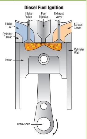
In the modern direct-injection diesel engine, fuel combustion is confined to a specially shaped region within the head of each piston. There, diesel fuel ignites spontaneously, yet in a carefully controlled manner. Old-style indirect-injection diesels were not capable of this precision. As a result, fuel efficiency suffered and emissions soared.
